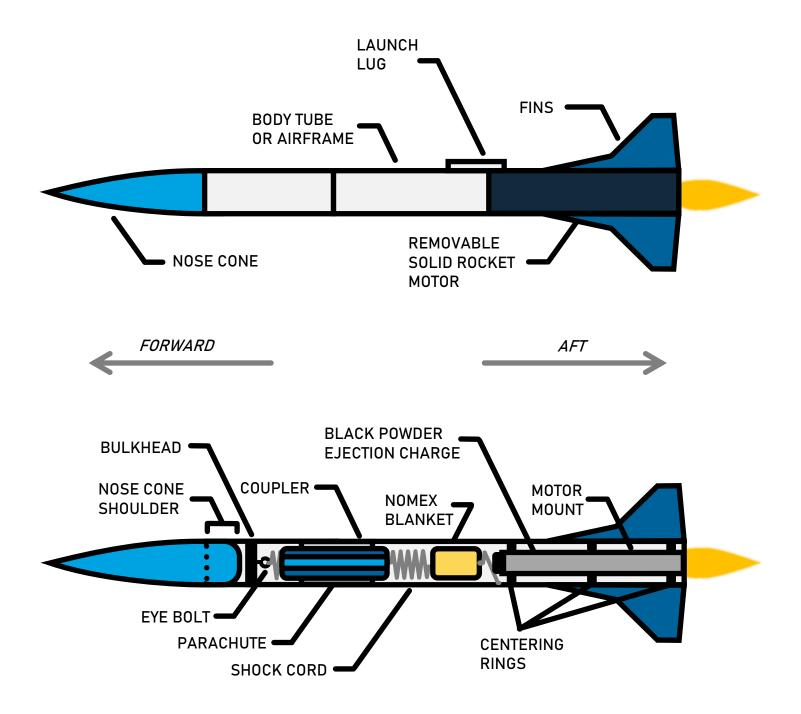
**NOSE CONE** - The top of the rocket, shaped so air will flow smoothly around the rocket. Nosecones typically follow a conical, tangent ogive, elliptical, or Haack shape.
